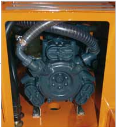
Diaphragm pump – maintenance-free, adjustable prewetting rate
